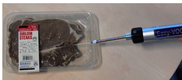
Figure 3: Sampling of the headspace of the packaged meat onto an inert-coated sorbent tube using the Easy-VOC grab-sampler.
