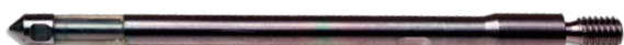
Figure 1: A standard-length (75 mm) HiSorb high-capacity sorptive extraction probe, showing the PDMS phase on the left.
